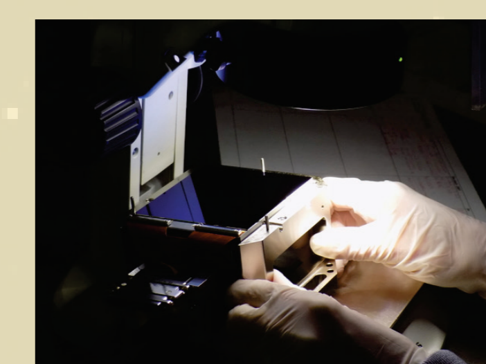
104 CCDs (4 CCDs per camera) 4510 x 4510 pixels Pixel size 18 μm – 15" on sky Built by Teledyne-e2v
